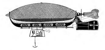
Screw propellers rotate in cylindical casings situated in the girder, and a fan, which is mounted on a universal joint at the stern of the balloon, directs a current of air against an adjacent surface. The said fan, it is stated, assists in propelling the balloon and the steering is effected by a double rudder operated by steering-cords.
